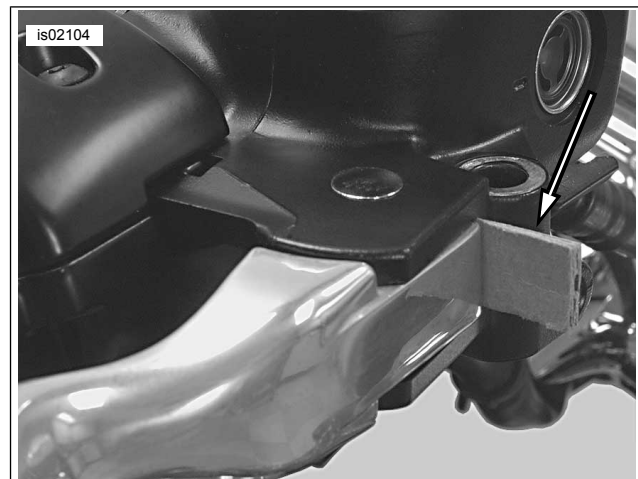
Figure 4. Install Cardboard Insert Before Removing or Installing Master Cylinder Assembly
