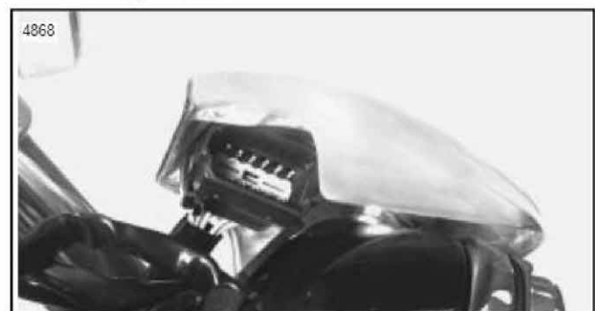
Figure 2. Unplugging 12-Place Connector (1995-1996 style connector shown)
