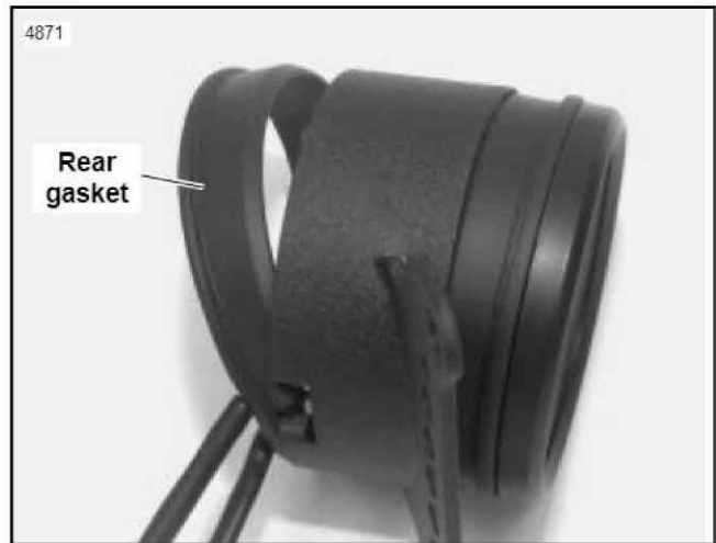
Figure 5. Removing Speedometer From Bracket
