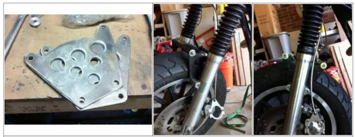
Home made fork brace constructed from two 1/4" steel plates, a hole saw, an angle grinder, some steel tubing and threaded rod. <sup>1)</sup>
