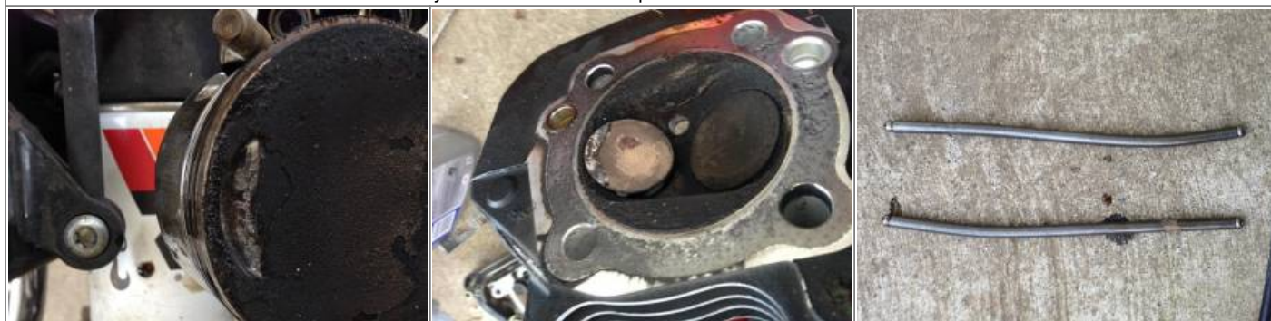
Heavy witness marks from piston contact with valve. 97)
