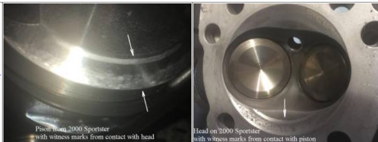
Light witness marks from piston contact with valve. 96)
