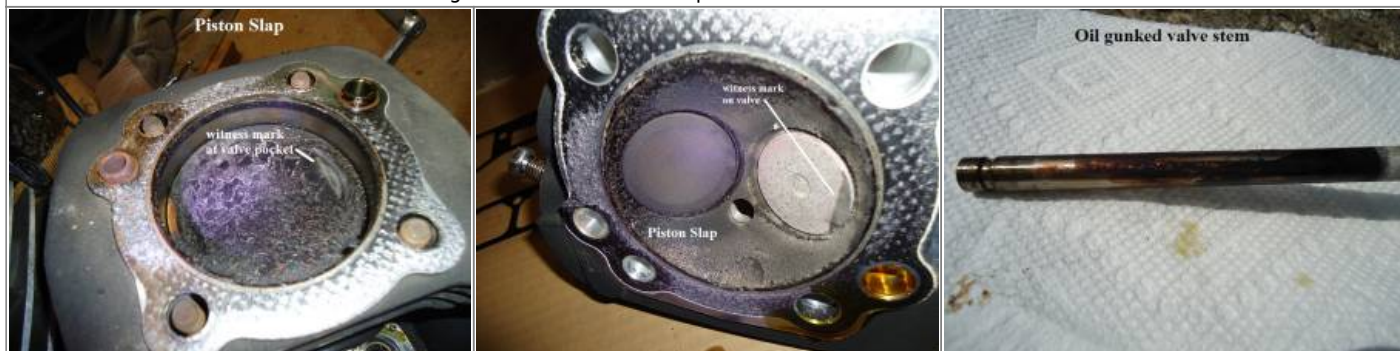
Heavy witness marks from piston contact with valve. 97)
