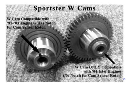
The #2 cam on the left is machined for the timing cup and therefore will work in 91-03 bikes. The #2 cam on the right can only be used in 04+ (crank trigger) bikes, unless someone does the machining.
