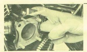
Install the manifold in the usual manner. We advise using teflon tape to cover the "O" rings before clamping. 1981 and up use band type seals. Install clamps lightly as manifold will require leveling. The standard leveling bracket is mounted from the center case bolt of the engine to the bottom left manifold hole, for later models mount in same position as stock mounted bracket.
