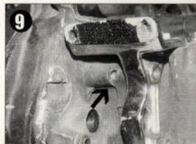
9 Be sure to check the rest of the case for cracks, too. This missing chunk (see arrow) should be replaced — by welding — but can easily be overlooked during a pre-purchase inspection.
