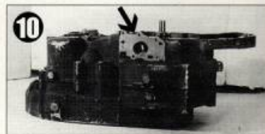
10 Don't forget to inspect the three drain holes on the bottom of the case. Give the oil pump surface (see arrow) a good look, too. A gouge or scratch here will give you an un-repairable oil leak.
