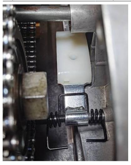
Finally, push the end of the spring up so it slides into the case as you push the cover home. The OEM Harley kit came with instructions that advise to check the gasket for clearance and trim it if necessary. I didn't have a problem with this James gasket.
