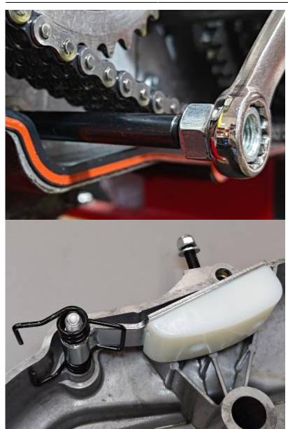
Here, the pivot stud is pushing the old bolt out while the spring and shoe stay in place.
