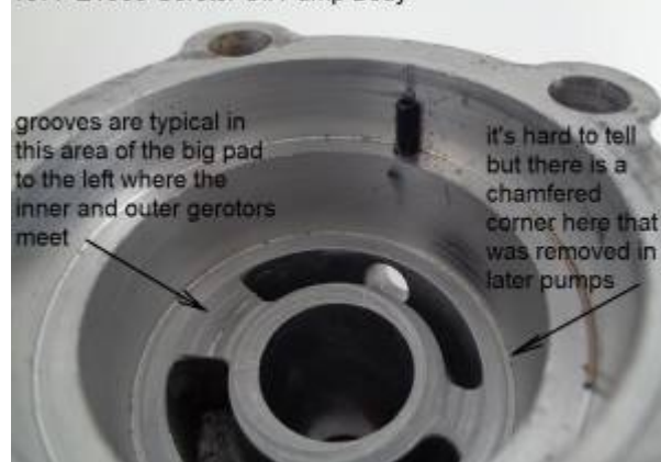
1977-E1983 Gerotor Oil Pump Body
