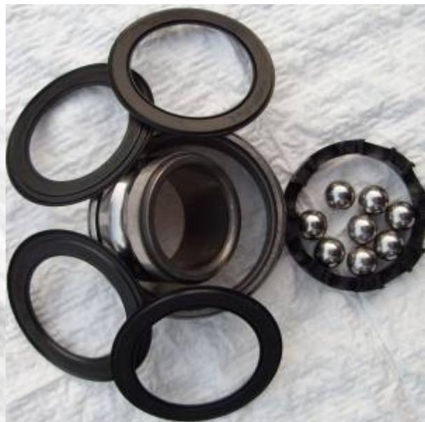
Multihdrdr goes on to say: "Besides being good quality bearings, I believe the seal arrangement contributes greatly to their longevity. The outer seal (on each side) is fixed to the stationary inner race and seals against the rotating outer race whereas the inner seal is fixed to the outer race and seals against the inner race with some grease between the seals. This creates a tough path for water and grit to arrive at the balls and races."
