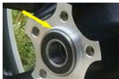
Installing 21mm-wide 4SSR bearing in 2008-later wheel (which has only 15mm-deep hub bearing cavity).
