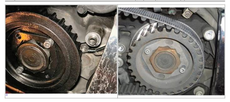
Pre-2004, on the outer flanged side, the center mounting splines are relatively flush with the flange face. But, on the engine side of the sprocket, the center mounting splines are recessed from the edge of the belt drive face. On 2004-later, the flange is on the engine side (with recessed splines there) and the mounting nut and lock plate are on the outer, flangeless, side.
