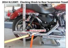
This is the side where I measure the axle height<sup>34)</sup> →
