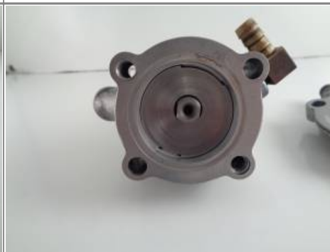
Separator Plate locked in place by pump body tabs 6)
