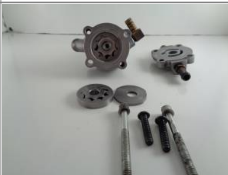
Scavenger Gerotors installed 5)
