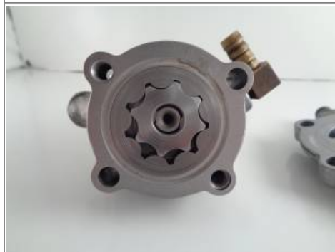
Feed Gerotors Installed 7)
