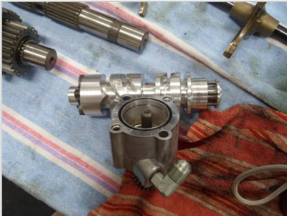
2005 Buell XB oil pump showing one of the two keys that prevent the separating washer from rotating. 4)
