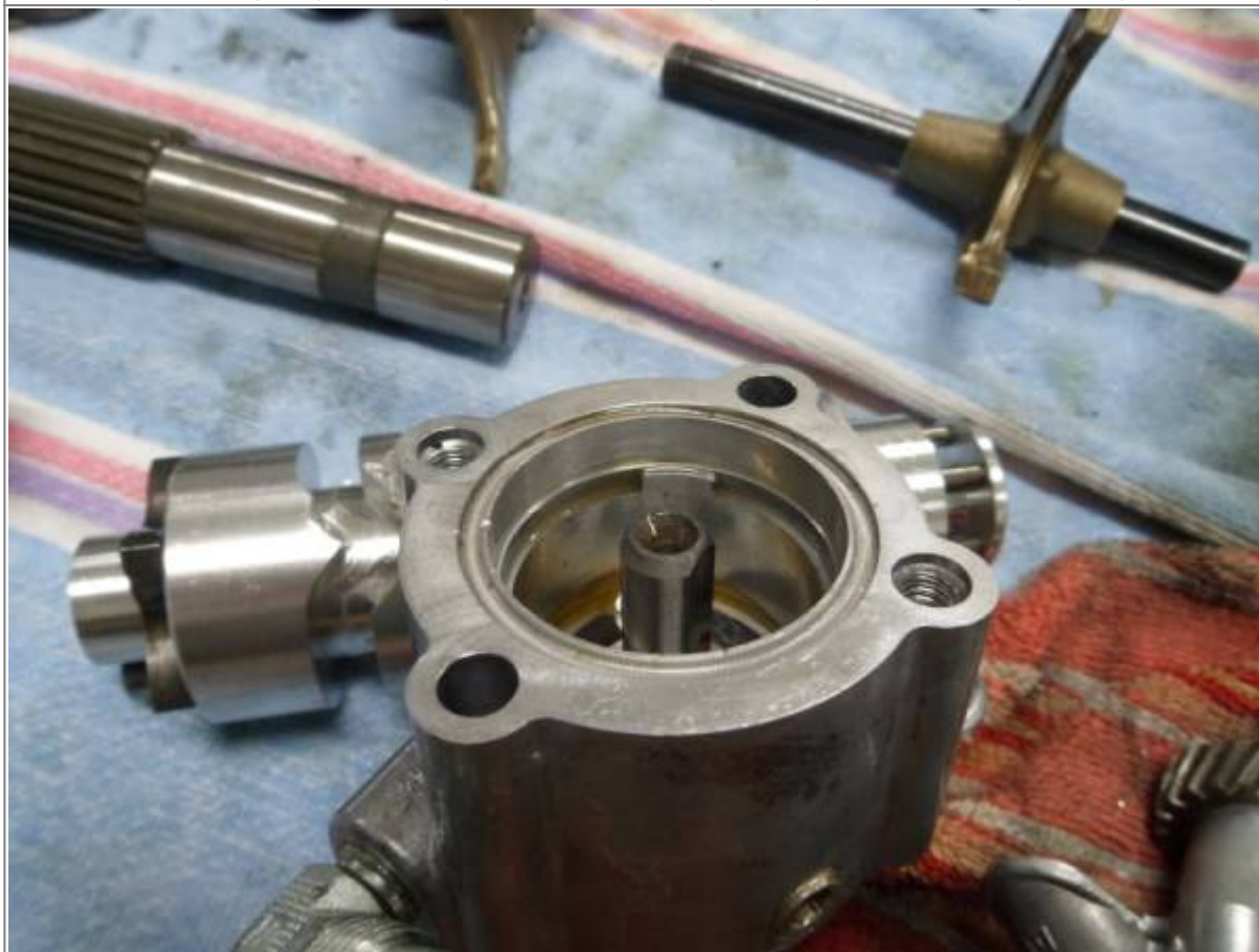
2005 Buell XB oil pump showing one of the two keys that prevent the separating washer from rotating. 4)
