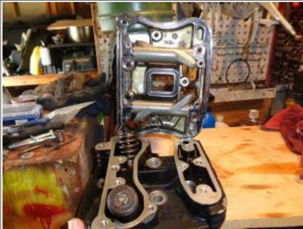
91-03 breather holes in the rocker box sections and head 13)
