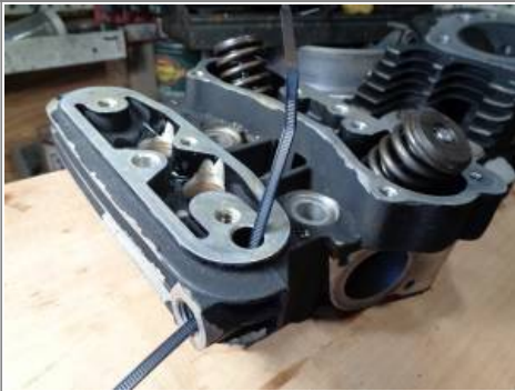
91-03 style front head drainage hole 14)
