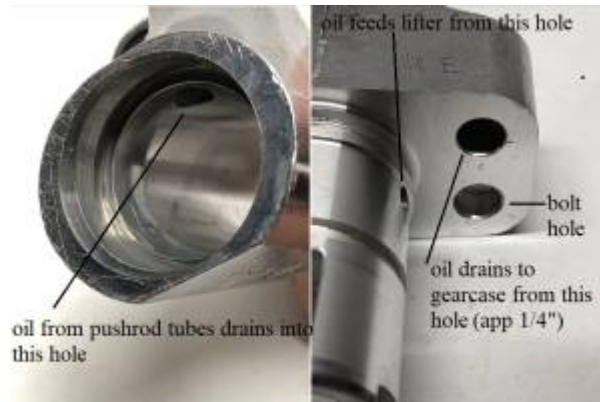
2) 1986-1990 Tappet Block Oiling (rear exhaust shown) 3)
