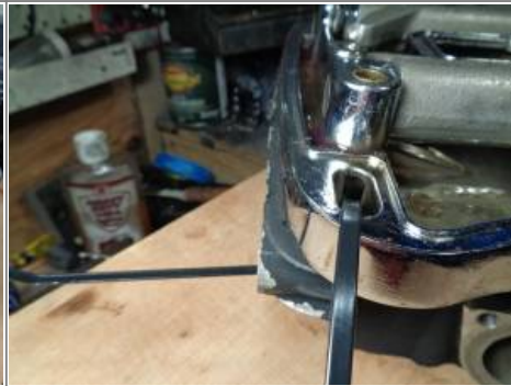
91-03 style front head drainage hole 14)
