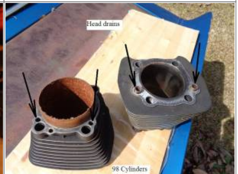
Head drains at the cylinder base on the case. 17)
