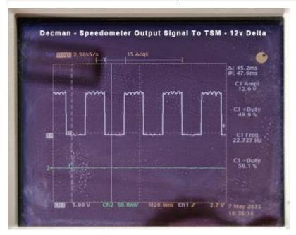
Electronic Explanation of the Vehicle Speed Sensor Function. (Reference XLForum Thread)
