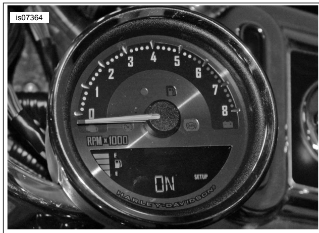
Figure 5. Fuel Level Display Setup
