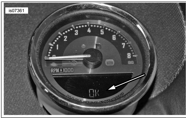
Figure 3. Speedometer Gauge Displaying "OK"
