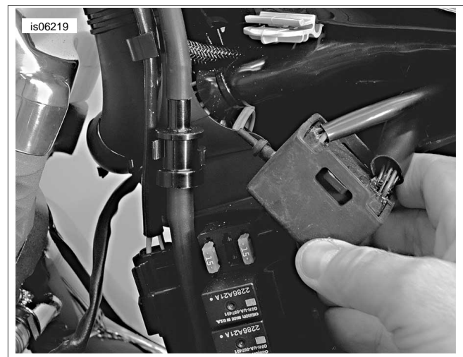
Figure 4. Converter Module Installation
