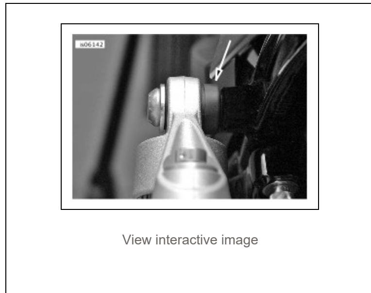
Figure 3. Install Thick Side Of Grommet To Frame Rail
