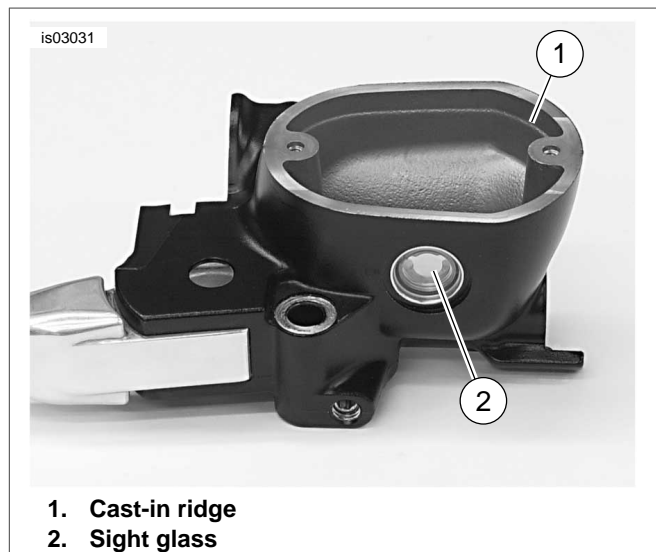
Figure 7. Filling Front Master Cylinder Reservoir
