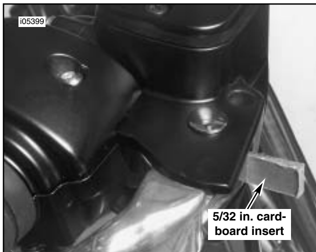
Figure 2. Install Insert Before Removing Master Cylinder
