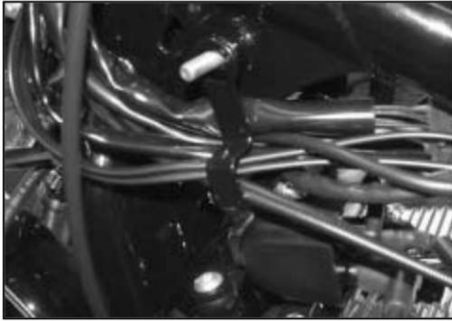
Figure 6. Throttle Cable Routing (2004 and Later XL models).
