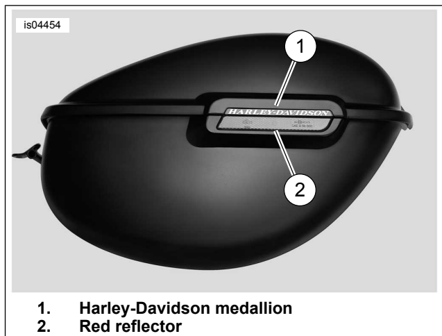
Figure 15. Install Medallion and Reflector
