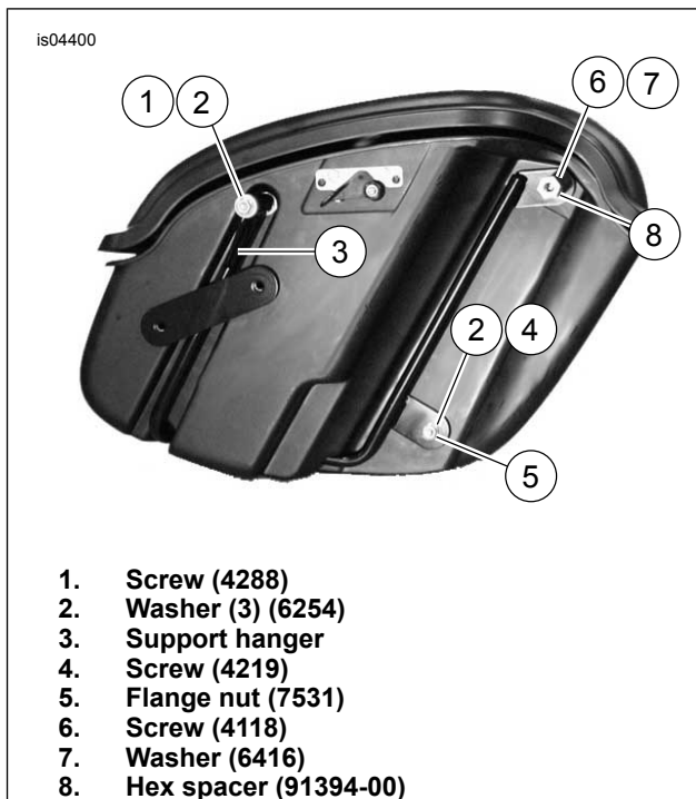
Figure 10. Assemble Support Hanger on Saddlebag
