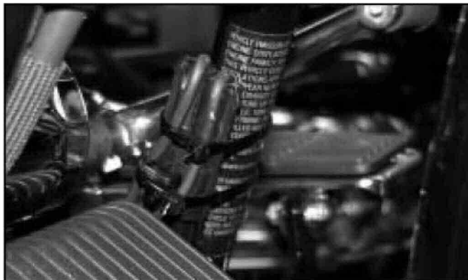
Figure 10. Secure regulator wiring with cable straps
