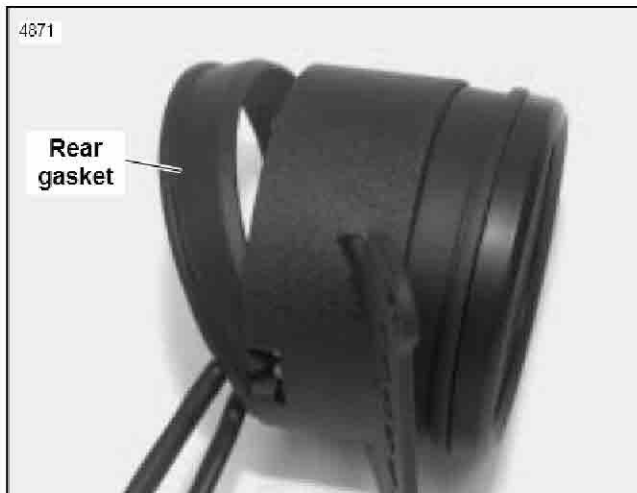
Figure 5. Removing Speedometer From Bracket
