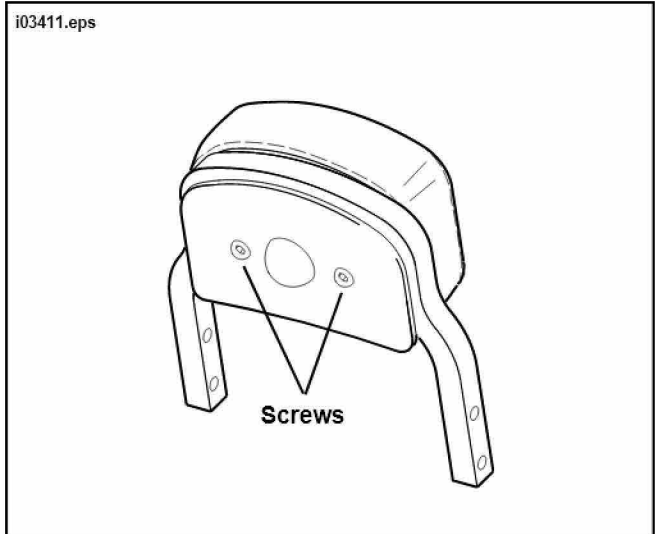
Figure 1. Backing Plate Installation
