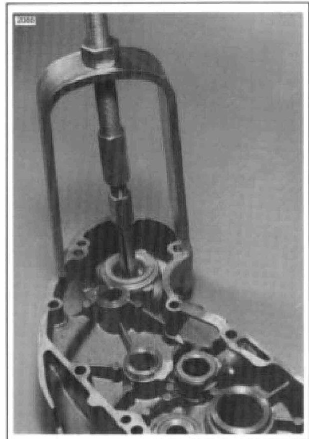
Figure 2. Early-Style Reed Valve Removal
