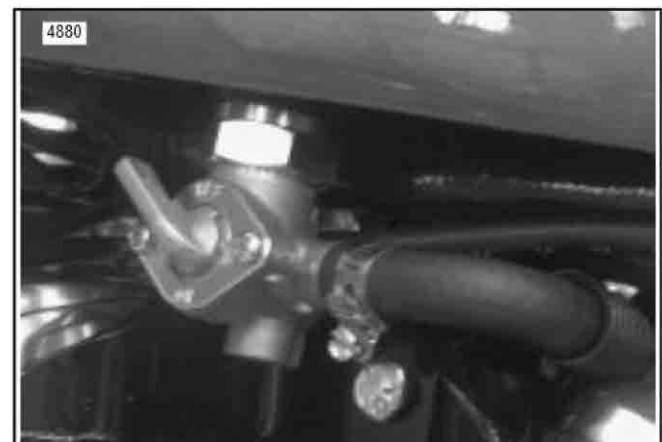
Figure 4. Fuel Valve And Hose location
