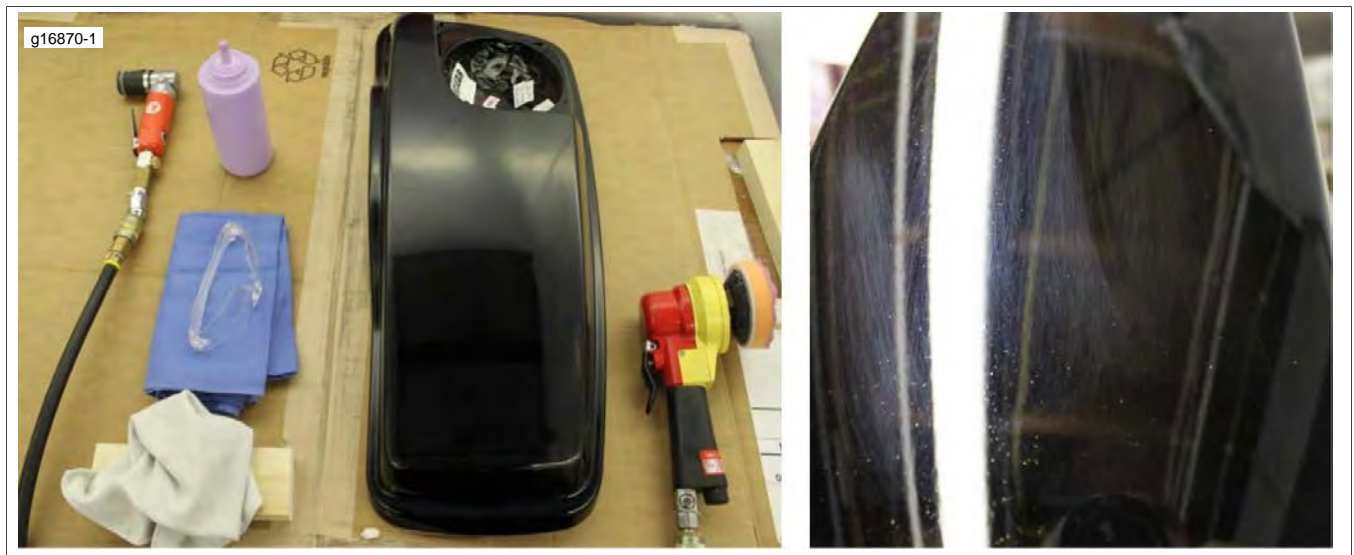
Figure 1. Preparation for Repair and Saddlebag Lid with Clear Coat Scratches
