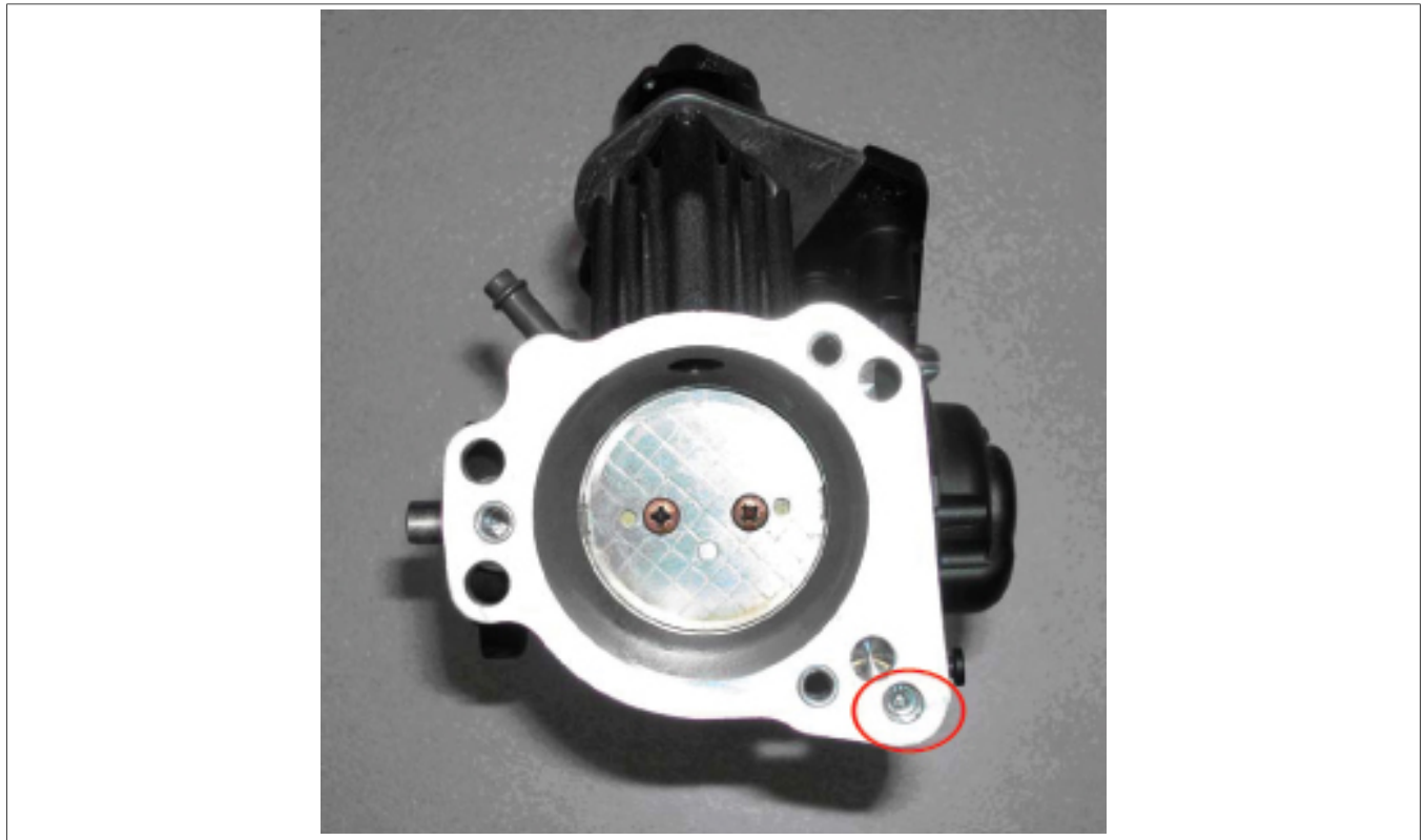
Figure 1. Induction Module and Throttle Stop Screw
