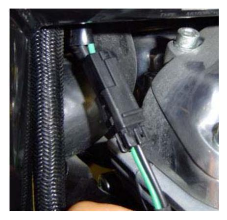
Although the wires are mismatched in color, the solenoid has no polarity and will operate regardless of how power is applied. No action is needed for this condition.
