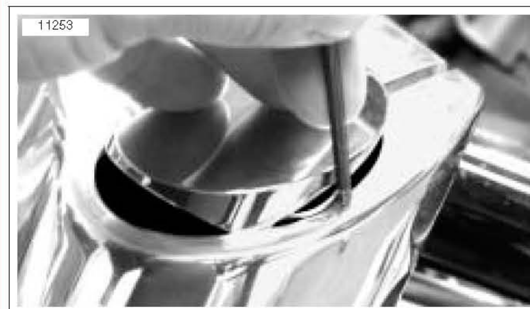
Figure 2-86. Install Fork Cap
