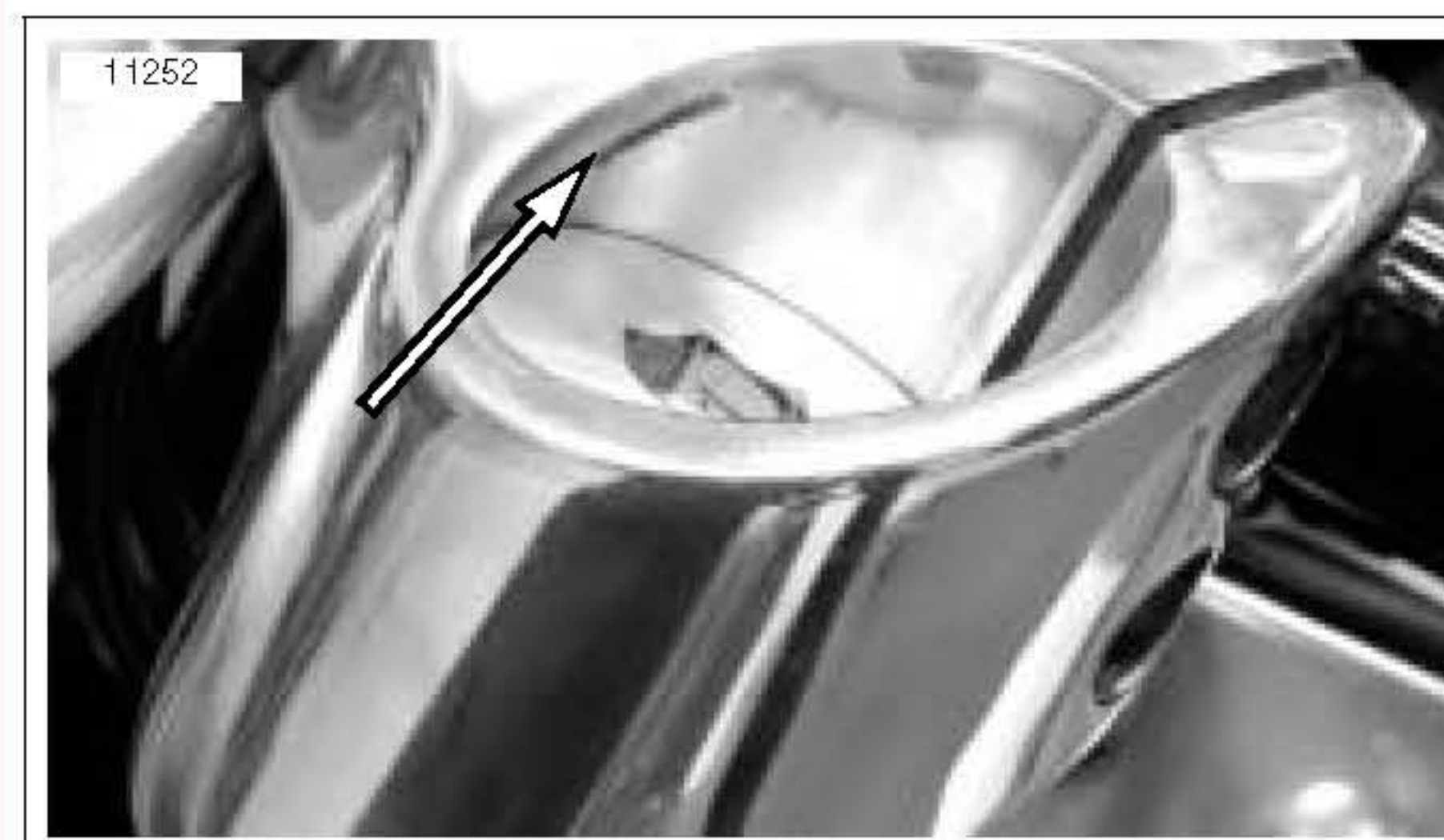
Figure 2-85. Notch In Upper Triple Tree
