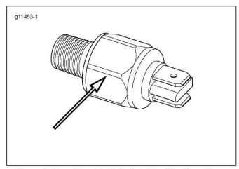
Figure 1. Rear Stop Light Switch Identification: Sharp Edges Are Removed On New Switch
