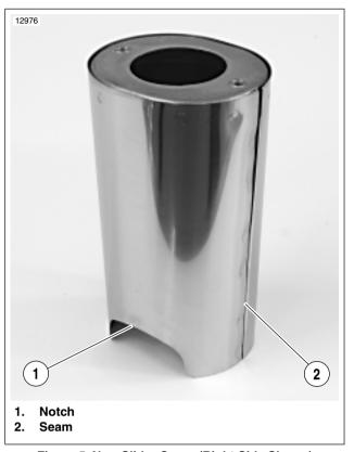
Figure 5. New Slider Cover (Right Side Shown)
