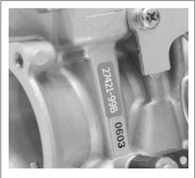
Figure 1. Install Silver “0603” Label on Carburetor
