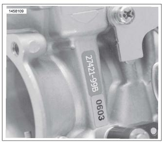
Figure 1. Install Silver "0603" Label on Carburetor (Optional)
