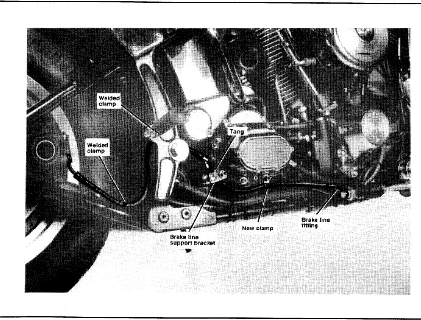
Figure 1. Replacement Brake Hose (Exhaust Removed For Illustration Purposes)
