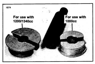
Figure 1. Bearing Race Tool
