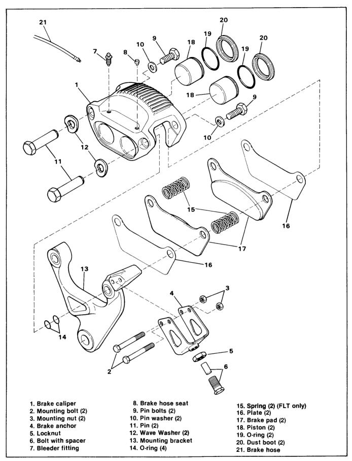
Figure 1. Rear Brake Caliper - FLT Shown
