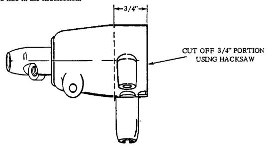
Install modified brake lever support on the handlebar and fit throttle grip assembly, part No. 45186-74P, snug against the support.
