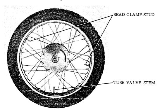
With hole in rim strip positioned at tube valve stem hole, assemble rim strip to rim, positioning it over bead clamps. With wheel assembly in a vertical position, push down on tire to allow access to align rim strip over spokes. Reinstall tube with valve stem located as shown.
