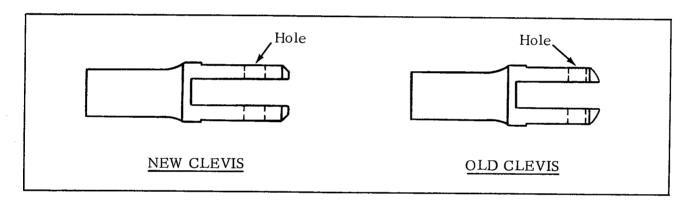
In compliance with the National Motor Vehicle Safety laws which apply whenever a safety hazard exists, we are required to have you install the correct brake rod clevis on all 1971 Super Glide motorcycles below Serial No. 20985 which are in your dealership area. This includes all motorcycles previously delivered to your customers, those on your floor or in transit.
