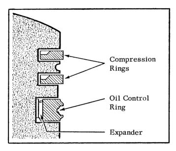
A two-piece oil control ring has been in use on the Sportster and Electra – Glide engine since the start of the 1966 model season.
