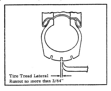
If tire tread runout is more than 3/64", remove tire from rim and check rim bead side runout to see if rim is at fault. (see sketch)
