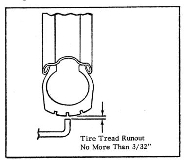
If tire tread runout is more than 3/32", remove tire from rim and check rim bead runout to see if rim is at fault, (see following sketch).
