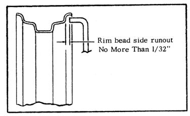
If rim side runout is less than 1/32", tire is at fault and should be replaced. If rim side runout is more than 1/32", correct by tightening selected spoke nipples as outlined in the service manual, reinstall old tire and recheck tire tread lateral runout.
