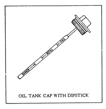
Oil tank holds 3 quarts with oil level at "FULL" mark. Do not fill above this level, as the tank needs some air space.
