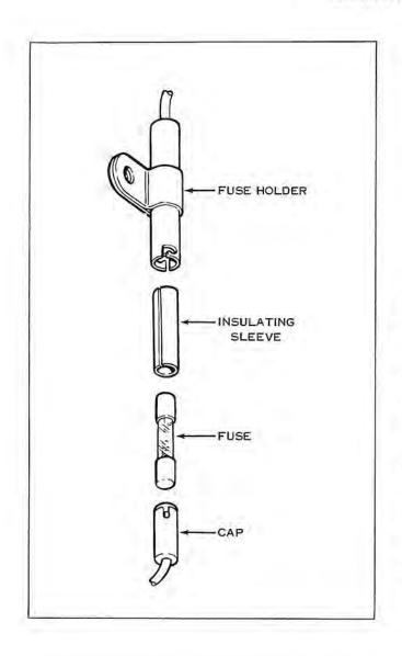
The following Harley-Davidson models have a cartridge type fuse in the generator field circuit to protect the electrical system.
