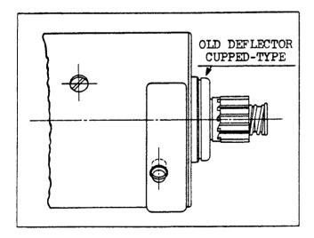
A change has been made in the generator drive end oil deflector of the 1958 fan cooled generator (Model 58R), used on radio-equipped Duo-Glide motorcycles and Servi-Cars. The illustrations show the new straight-type oil deflector and the old cupped-type oil deflector installed on the generator drive end.
