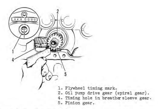
Figure 1. Timing Crankcase Breather
