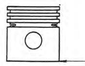
All Models except 125 c.c. Models and 165 c.c. Models -piston should be fitted .001" to .002" clearance in cylinder, checking fit at bottom of skirt, front to rear.
