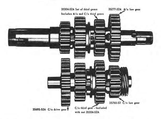
Five of the transmission gears supplied for servicing 1952-53 K transmission have been made much stronger gears as a result of modification of teeth, and changes in material and heat treatment. (These five gears are indicated in illustration.) The other three gears applying to 1952-53 transmission have not been changed. These three gears are:
